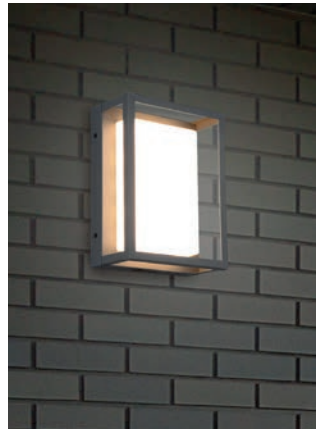
LED-Fassadenleuchte Metall anthrazit B 180, H 240 inkl. 1xLED/10,5 W/1100 lm/ 2300/3000/4000 K DIP-Switch
